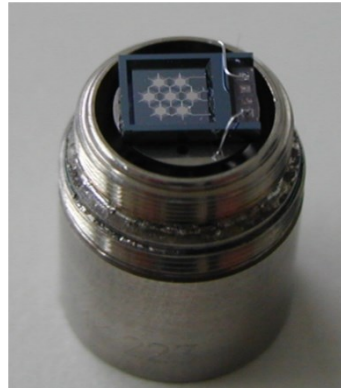
CMUT assembled on 1/4 " capsule or characterization
