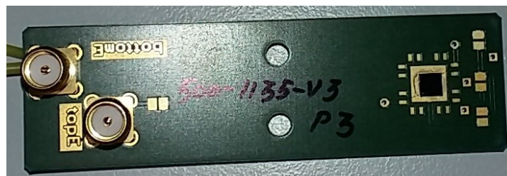
CMUT on test PCB
